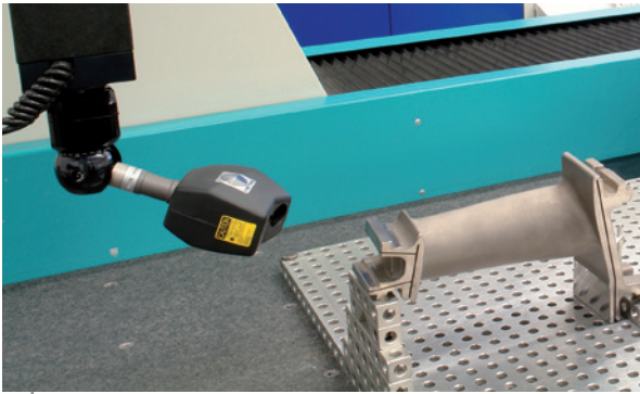
On average, a blade is inspected in a few minutes, including repeated scanning of its linear notches under different angles.
